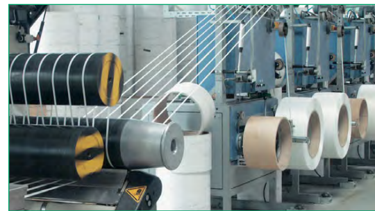
Fig. 4 Stretching process of Secugrid® ribs
