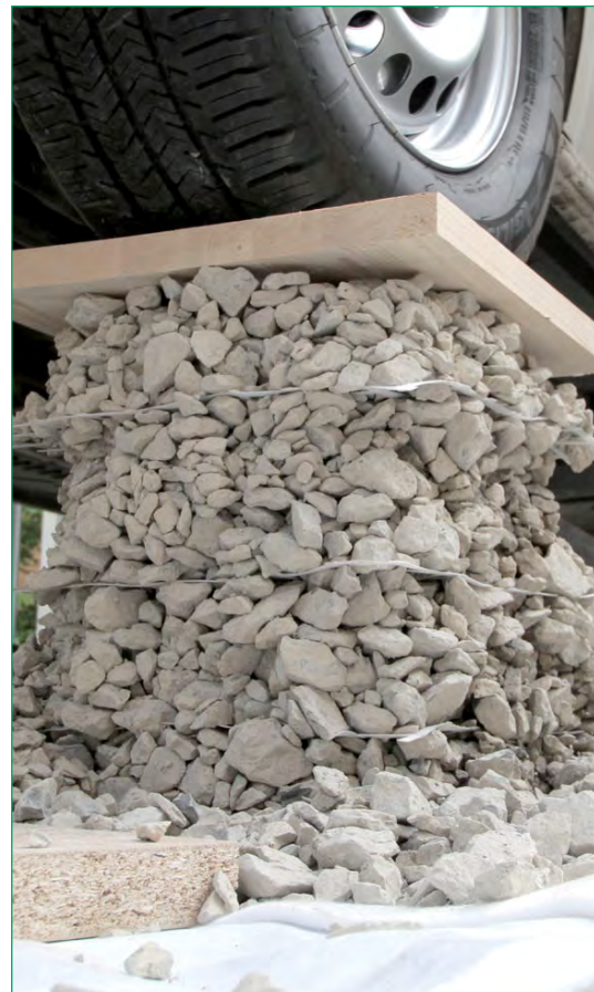
Fig. 10 Demonstration of the interlock effect with a car standing on a Secugrid® rein- forced gravel column
