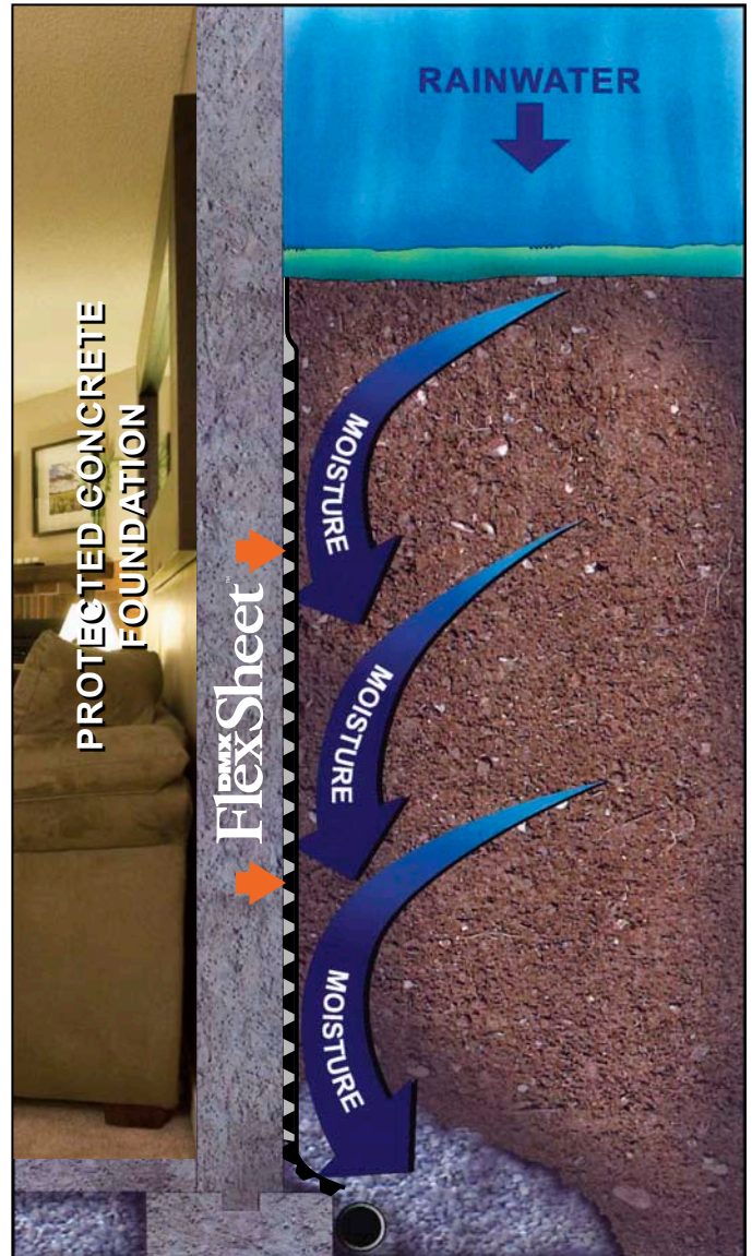
DMX FlexSheet™ applied to foundation wall eliminates the effects of Capillary Suction and Hydrostatic Load.
